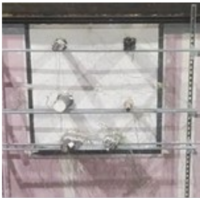
Preinsertion and insertion of FZ400 in larger seal (Up to EI120, service dependant)
